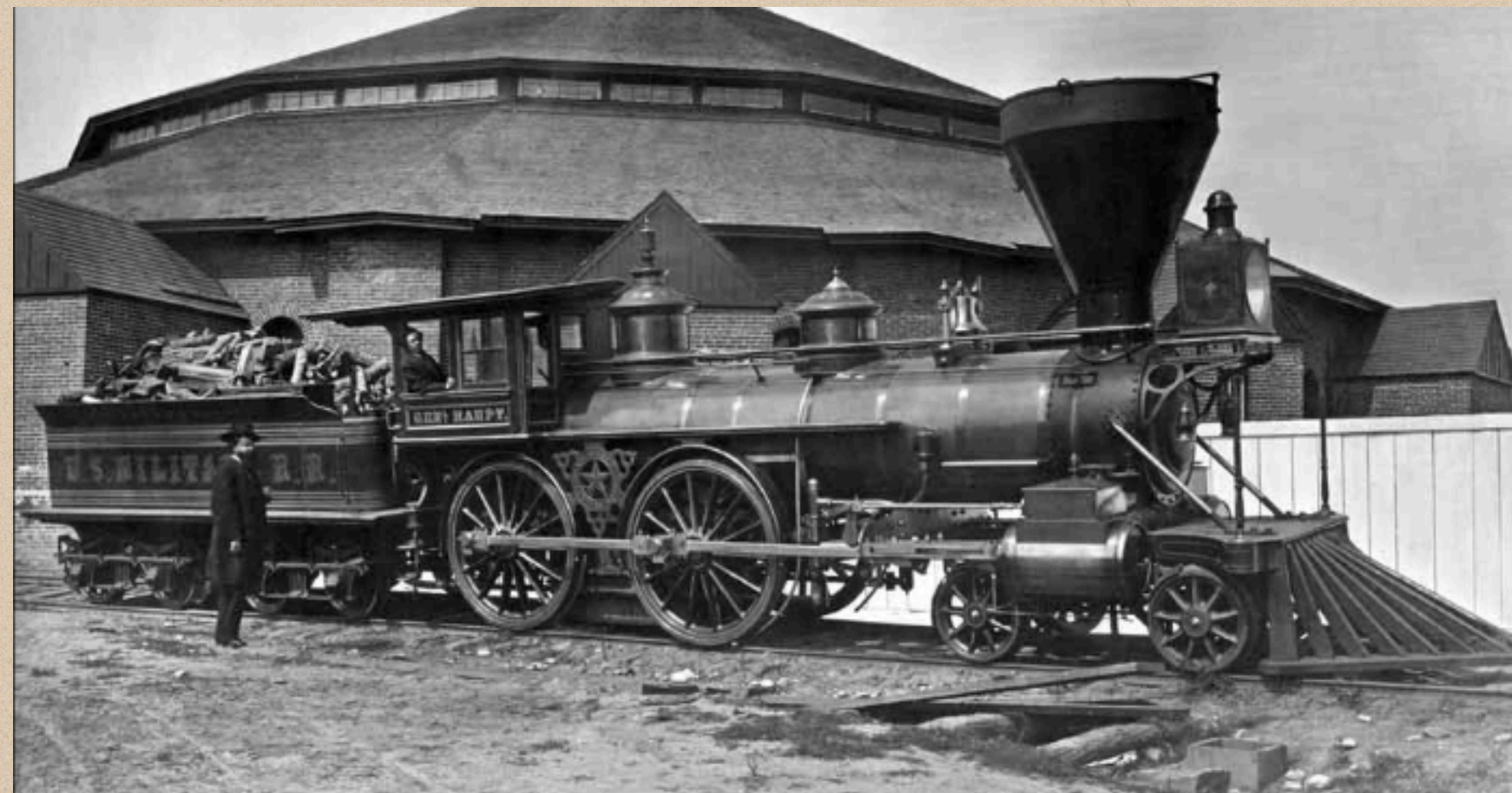
The wood-burning 4-4-0 locomotive Genl. Haupt at the Alexandria, Virginia, roundhouse
